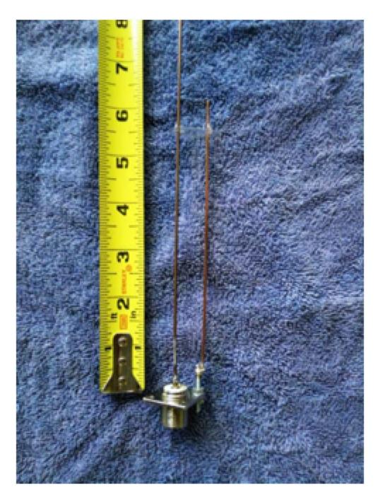
For dual band operation add three 20 Inch radials to the unused S0-239 holes.
