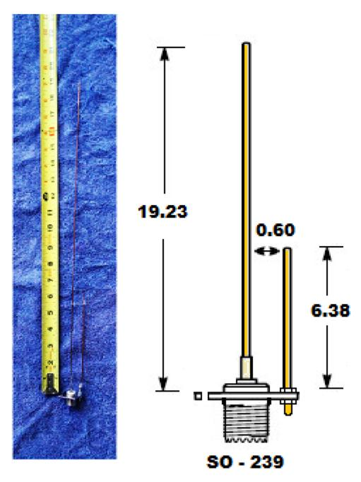
The key step in making this antenna is spacing the elements 0.60 Inches as the SO-239 spacing is closer to 1/2 Inch. Construct an eccentric or off-center connection using a 6-32 screw and solder the side of the screw to the side of the welding rod to form the 1/4 wavelength element. See detail in picture below. This arrangement provides to adjustments; spacing can be varied by rotation to get the 0.60 Inches and fine tuning of the 6.38 Inches with the vertical screw position.
