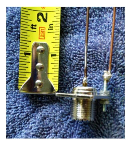
A common problem with small antenna elements is maintaining the spacing between the elements as the 1/16 Inch Rod is easily bent. Adding a plastic spacer about five inches up the elements with a drop of RTV silicone works great. See detail in picture below. In fact I have found a good use for the indestructible plastic packages used for display packages. Just cut a  $1 \times 1/2$  Inch plastic scrap and drill two holes spaced at 0.60 Inches.
